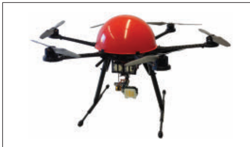
▲ Fig. 1 Hexacopter UAV equipped with a radar/gimbal combination for target tracking.
